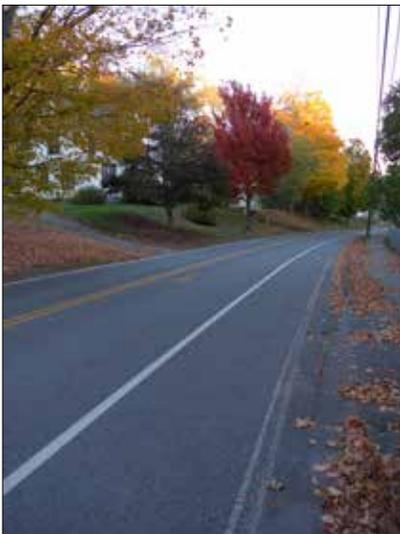
← Even though this road striping does not make regulation-width bike lanes, it does slow motorized traffic and leaves a wider shoulder for bikers and pedestrians. Bangor Trails has been working with the City to stripe wider shoulders to make Bangor more bicycle-friendly. Send us your photos of striping you like, and send us photos of places that need to be made more bicycle-friendly too.
